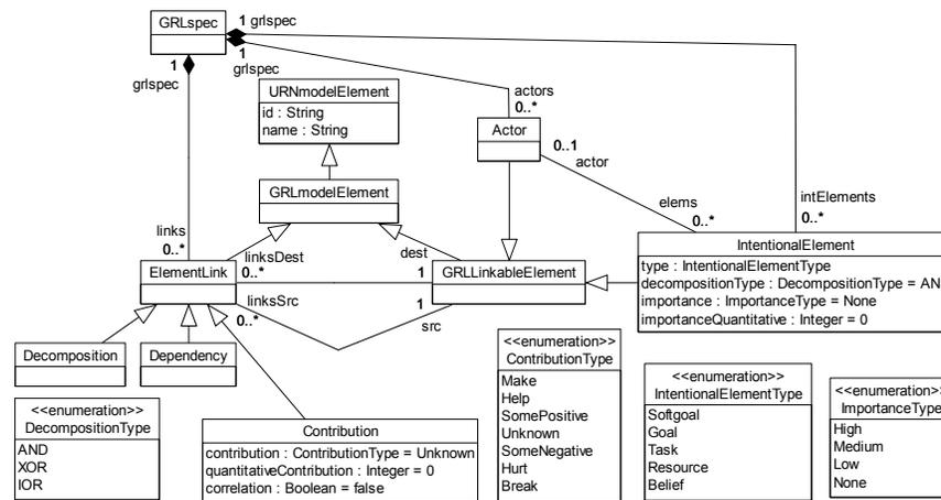
Fig. 2 GRL Metamodel – Core Concepts (from Z.151)
