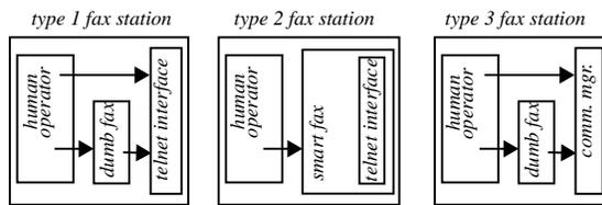
through a telephone network. A type 1 fax station is a human operator and a dumb fax machine interacting through an ordinary telephone handset. A type 2 fax station has a smart, software-controlled fax machine that itself provides the interface to the telephone network. A type 3 fax station is typified by a home office with an ISDN connection in which a software-controlled communications manager controls interactions over the circuits provided by the telephone company.
