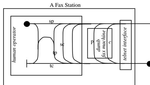
the chosen internal configuration of the fax station (shown here is a binding for type 1 fax stations). Choosing a type 2 or type 3 fax station would require assigning the setup and teardown responsibilities to internal software components of the black boxes. There is nothing new at the use case map level in doing this.
