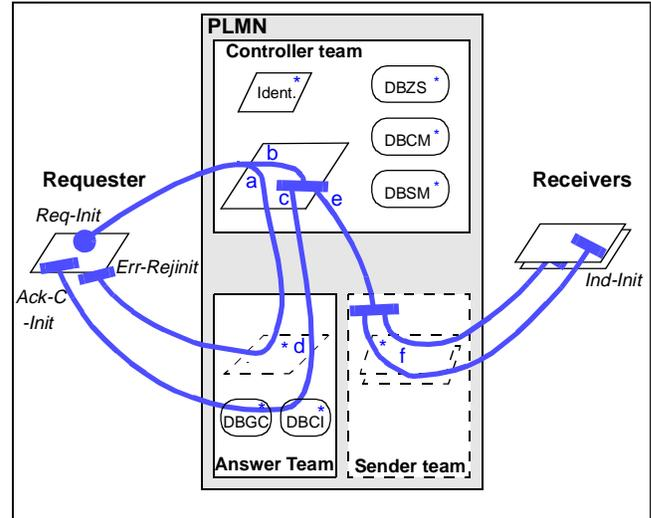
Additional information on the responsibilities is provided in Table 1. At this point, it is possible to detail their type (request, error, acknowledgement, indication, condition, or internal activity), parameters, allocation to a component, and additional comments. Conditions can be refined more formally once the data types and data structures are known.
