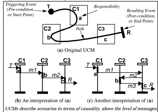
A causal relationship can be refined in many ways in terms of exchanges of messages, depending on the components structure, the available communication channels, and on the chosen protocols. Several MSCs could be considered as valid implementations of a UCM. For example, the MSC in Figure 1(b) represents a straightforward interpretation of Figure 1(a). The MSC in Figure 1(c) could result from an architecture where there is no channel directly linking **C<sub>1</sub>**
